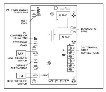
Figure 24. Outdoor Unit Defrost Control (CMC1)
